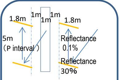
The light-receiving panel on the front side has a reflectance of 30% (half mirror) and the back side has a reflectance of 0.1% (anti-reflection coating) to increase power generation efficiency on the back side, which is less likely to reach high temperatures. Also, the best shift amount is automatically set according to the angle of the sun.
