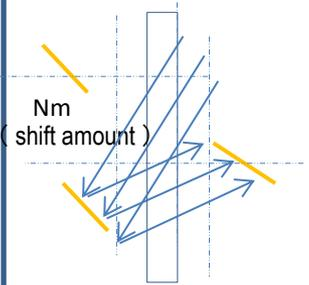
When the position of the sun becomes lower, the angle and shift amount of the solar panels are automatically determined so that the front reflected light from the second row of solar panels reaches the rear surface of the first row.
